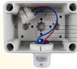
Multimeter Points Gain Potentiometer 4-20mA Signal (Blue) +24V DC (Red) Zero Potentiometer
